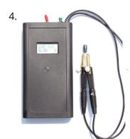
ATMEGA8 FT232R USB ESR METER CIRCUIT USB ESR Meter Circuit The main part of the meter is a ATmega8 microcontroller that controls the entire device. Its main the task is to process measured data and perform...
