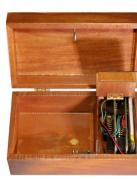
Box with a Music Lock using ATMega328P Microcontroller There are a lot of locks out there. There are locks open with a key, with a combination of digits, with various bodily parts, or with a correct geolocation. I...
