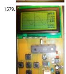
Low speed AVR oscilloscope V2.00 (Is updated on 19 Mar 2011) >> The firmware was updated on 19 Mar 2011 << A few months ago a friend of mine -c mechanical at profession- told me that he had problem with some car sensors. He couldn't check, with a simple multimeter, if a sensor was working p ...... Listed under: AVR ATmega Projects, LCD Projects, Metering - Instrument Projects
