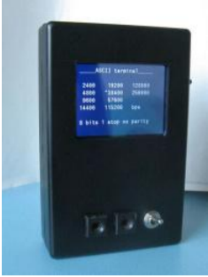
Serial Monitor With ILI9341 and BluePiII Serial (ascii) monitor with 9 lines of 28 char. Baudrate from 2400 up to 256000 baud. Digital 3.3V or 5V input. Powered by a single Lithium-Ion battery. (3.7V nominal) Supplies: ILI9341 display (here a parallel version is used) BluePiII (or other board with a STM32F103C8) 74HC14..... Listed under: Battery Projects
