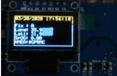
GPS Monitoring With OLED Display Project Hello everyone, in this quick article I will share with you my project : ATGM332D GPS module with SAMD21J18 Microcontroller and SSD1306 OLED 128*64 display, I built a special PCB for it on Eagle Autodesk, and program it using Atmel studio 7.0 and ASF4 so in..... Listed under: GPS Based Projects
