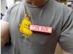
Bluetooth On "Air" Lapel Pin I was working on an unrelated project that utilizes Bluetooth, I had to test the communication so I built one of the Arduino test circuits. The light contains all of the electronics, microcontroller and battery which can be recharged VIA USB. It uses really strong..... Listed under: Other Projects
