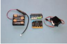
WaveShare Motor/Servo Driver With Micro:bit This Instructable will show you how to use a WaveShare motor/servo board with a micro:bit to power multiple servo motors. This board will make it possible to run more powerful servo motors than the micro servo motor that you can run directly from the micro:bit..... Listed under: Motor Projects
