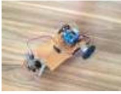
Obsatcle Avoidance Vehicle Using ATmega328P Microcontroller (Arduino) Obstacle Avoidance Vehicle capable of detecting objects, scanning the area and navigating through the less obstructed path. Step 1: Materials Needed Hardware Arduino UNO based on ATmega328 microcontroller DYP-ME007 ultrasonic sensor Servomotor L298N...
