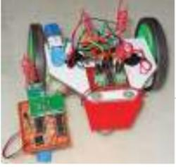
Wireless Gesture Controlled Robot Using Micro-controller ATmega328 In this wireless gesture controlled robot project I am going to control a robot using hand gestures. This is an easy, user-friendly way to interact with robotic systems and robots. An accelerometer...
