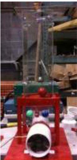
Ultrasonic Spheroid Levitation Device Using Atmega16 Introduction The goal of this project was to design and build a gaming device capable of levitating a ping pong ball at varying heights based on the proximity of the...
